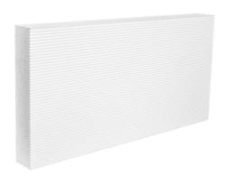
Unstressed insulation panel suitable for external thermal insulation systems, made of white conventional sintered expanded polystyrene (EPS), with external grooved pattern to improve system impact resistance. TERMOK8 A.R. Max 20 J and 60 J.
